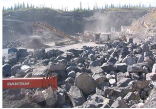
figure 22. Excessive dust caused by crushing operations can be mitigated by spraying water or using dust skirts on conveyors.
