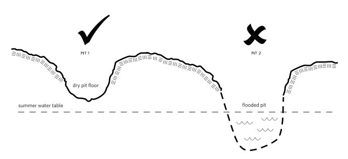
figure 13. Ensure pit excavation is well above the summer water table. (Redrawn from Robertson and Brandt, 1997, p. 31.)
