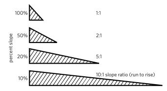
figure 18. Slopes can be expressed as a ratio of the horizontal run over the vertical rise, or as a percentage. (Redrawn from Robertson and Brandt, 1997, p. 47.)
