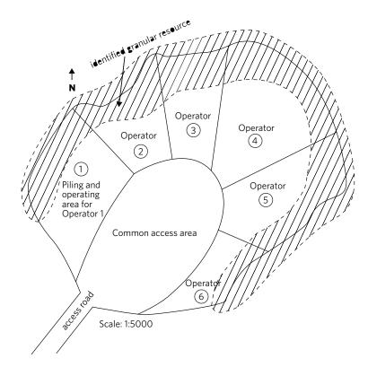
figure 15. Planned site layout for a multiple-user pit.
