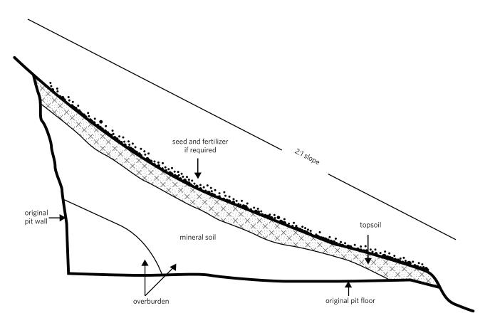
figure 26. Proper placement of overburden, mineral soil and topsoil for reclamation. (Redrawn from Robertson and Brandt, 1997, p. 42.)
