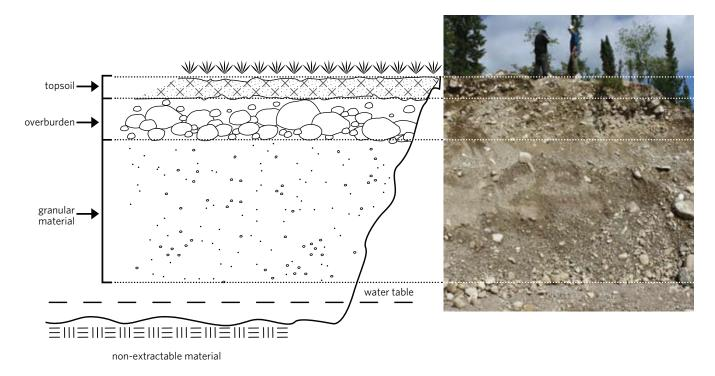
figure 19. Typical stratigraphy of a pit or quarry site showing topsoil and overburden layers over granular material.
