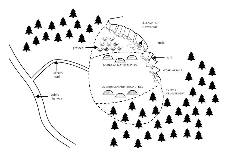
figure 9. A pit that is being progressively reclaimed during operations.
