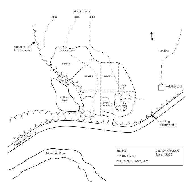
figure 14. Site design diagram to be submitted with a pit/quarry development plan. (Redrawn from Robertson and Brandt, 1997, p. 64.)
