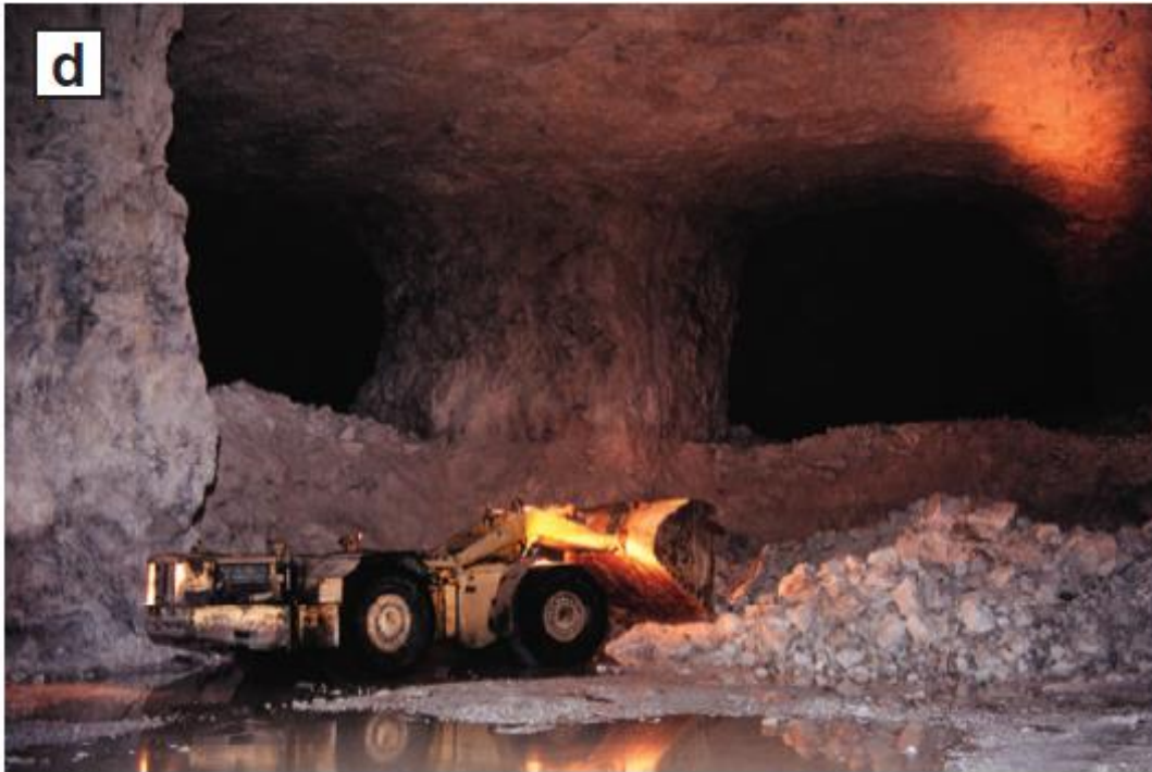
Scoop tram close to one of the spodumene zone pillars illustrating the room and pillar method used at Tanco.
